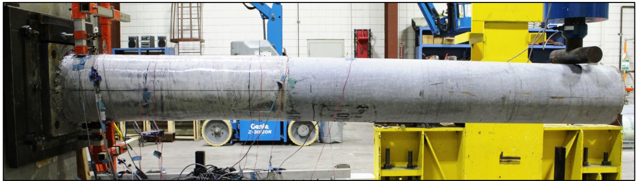
(a) Displaced shape of pole
