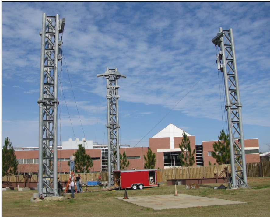
Figure 236. Impact pendulum at Structures Research Center in Tallahassee (IM-2 on pedestal)
