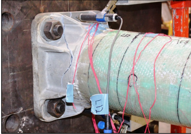
(a) Fractured base plate and sleeve
