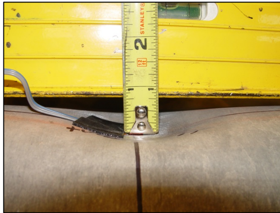
Figure 55. ALu-1.b laboratory-applied dent
