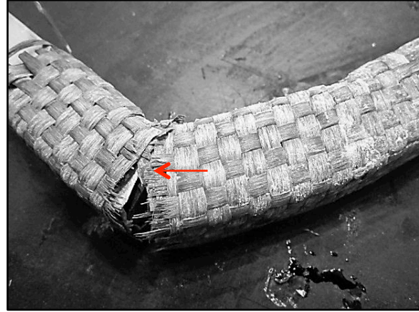
Figure 23. Substrate and FRP rupture
