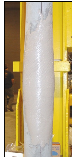
Figure 13. Sikadur 31 dent fill 2
