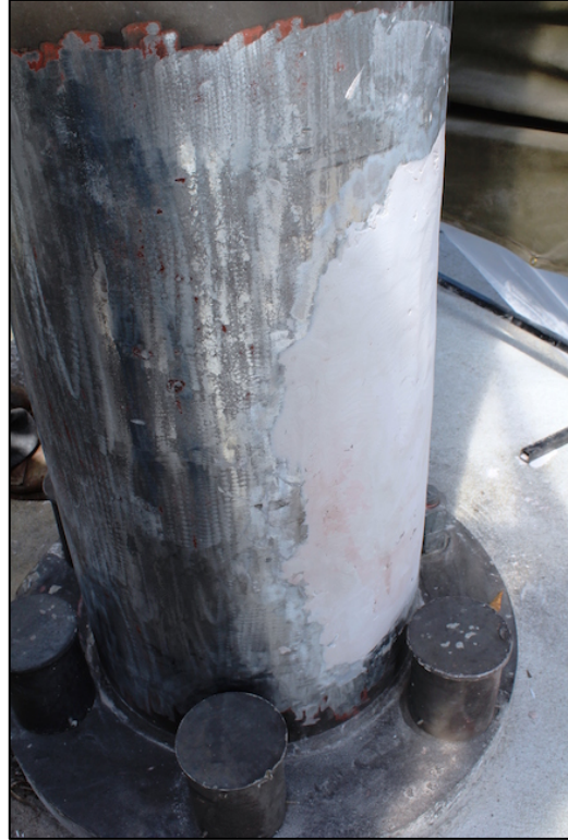
(b) After dent filler application and sanding
