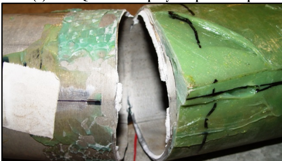
(c) Aluminum rupture
