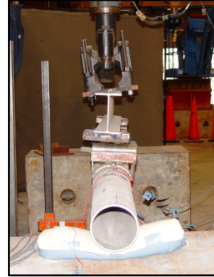
(b) Flange buckling of load spreader beam
