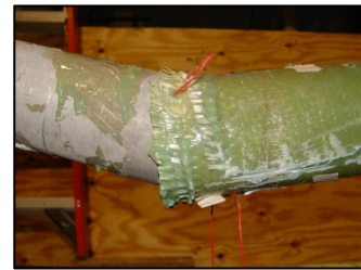
(c) Rupture joint
