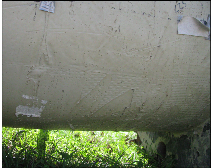
(b) Slight dilation of cross-section in the region of the dent
