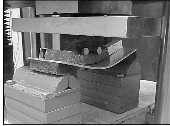
Figure 17. FRP compressive test, under loading
