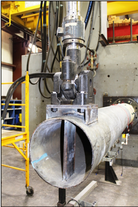
Figure 206. Fatigue test actuator connection with stiffener at end section
