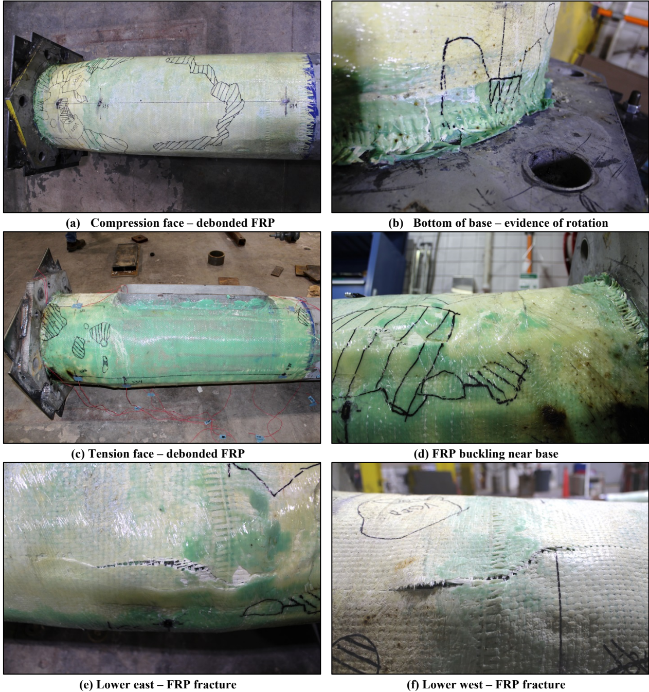
Figure 176. ST-6 failure modes
