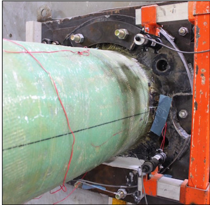
Figure 207. Fatigue test connection to buttress with plate washers on top and bottom
