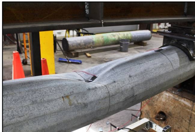
Figure 79. STu-1.f failed pole section
