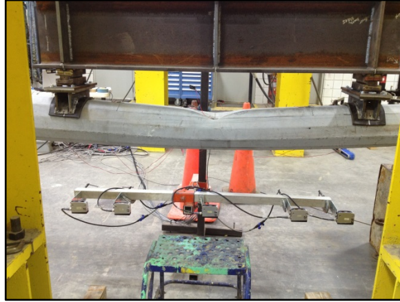
Figure 76. STu-1.e failed section
