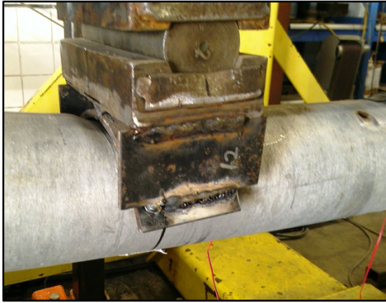
Figure 61. ALu-4.a local buckling at load applicator
