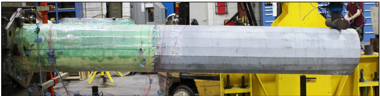
Figure 175. ST-6 deflected shape at failure
