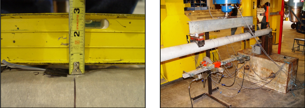
Figure 52. ALu-1.a laboratory-applied dent and test configuration
