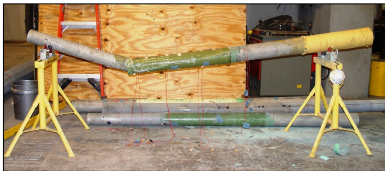
(b) Aluminum rupture failure
