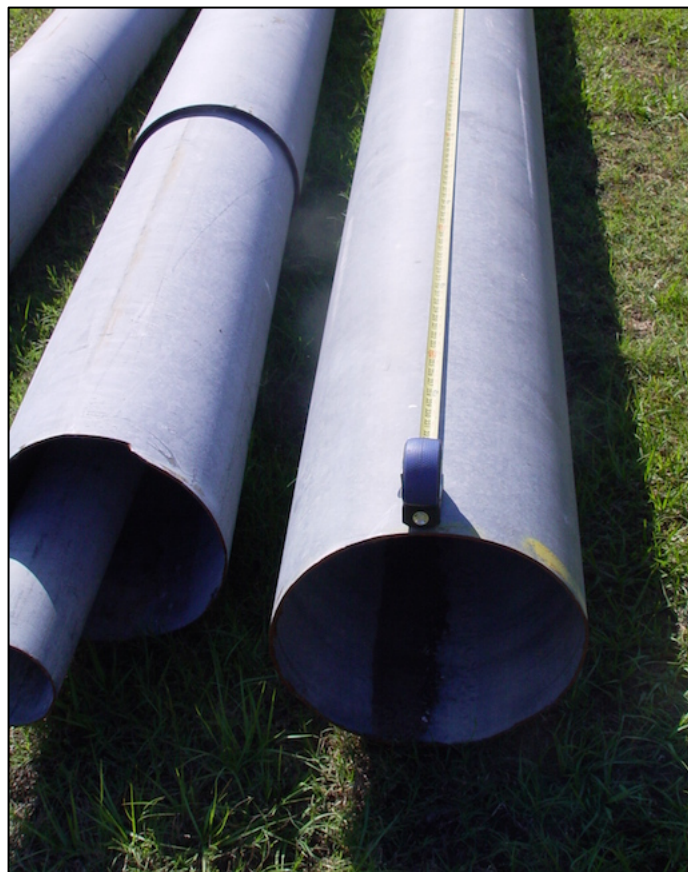
Figure 44. Pole specimens located in the yard prior to cutting for the component-level tests
