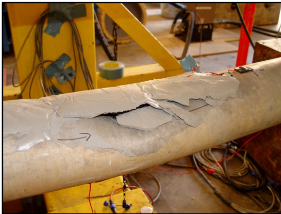
(a) Compressively-failed epoxy fill
