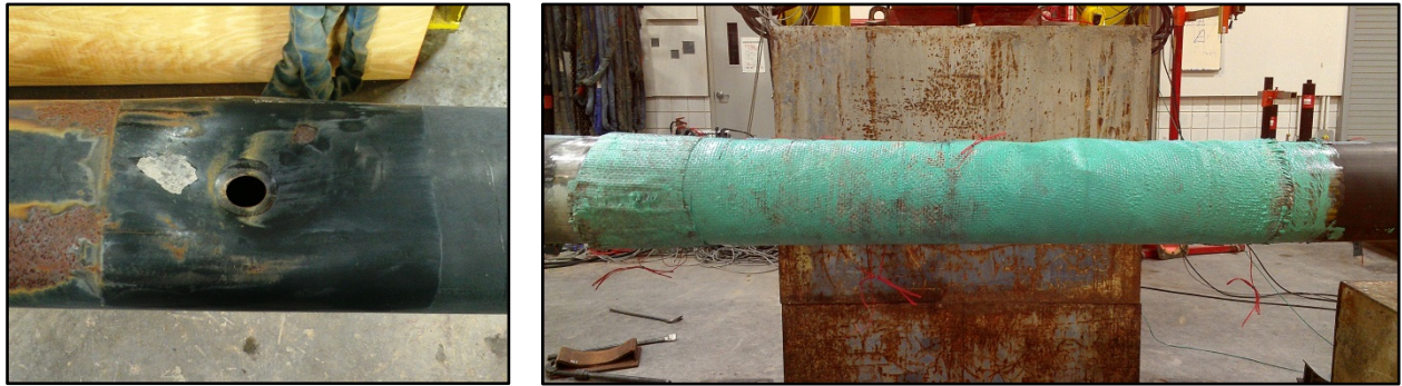
(a) STw-4.c dent over button opening (b) STw-4.c composite wrap Figure 109. STw-4.c dent and composite wrap
