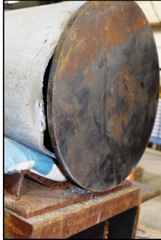
Figure 68. STu-1.b end weld failure
