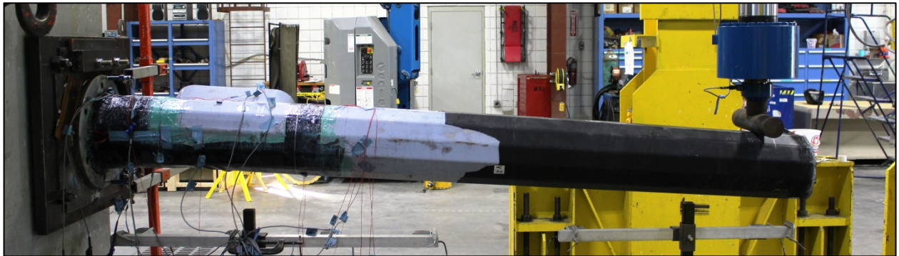
(a) Deflected shape of pole during loading
