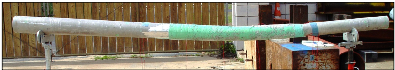
Figure 100. ALw-7.a displaced shape
