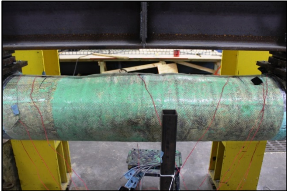
Figure 107. STw-3.b repaired section in test setup
